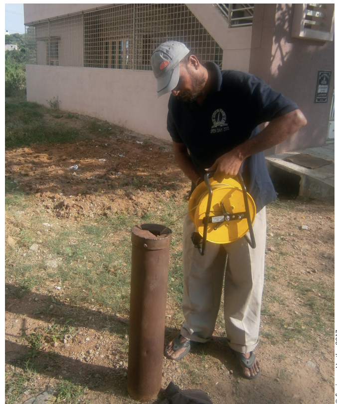
P. Giriraj, a research field team member from the Indian Institute of Science, measures water levels from an abandoned borewell in south-west Bangalore.
